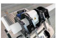
The newly designed planer and heating element are arranged in a way which ensures full 360° visibility and access to the welding area for complex isometrics.
