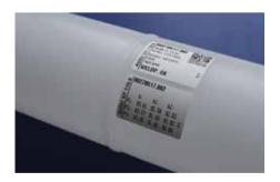
"Ongoing job report" on the machine, QR code and mobile AGRU app record all welding parameters, such as temperature, joining pressure and time.
