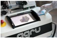
RFID data input for system access and welder identification in combination with the pre-programmed welding processes ensure a very safe and automatic welding process.
