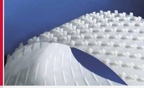
The innovative structure enables a fast removal and avoidance of deposits during the transport of media. The concrete protective liner with bionic surface provides a remarkable self-cleaning effect, even at low flow capacities. Additionally the surface structure improves the footing (works like a slip-and-slide protection) and thus the safety in the channel.
